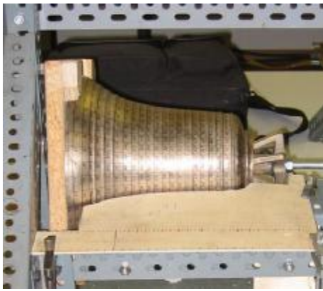
External measurement grid
