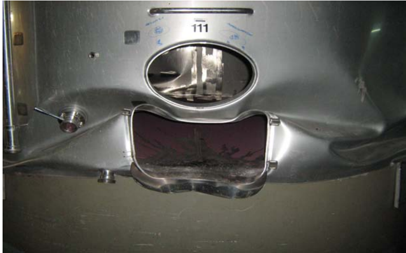
Figure 3. Failure of the cleaning doors.
