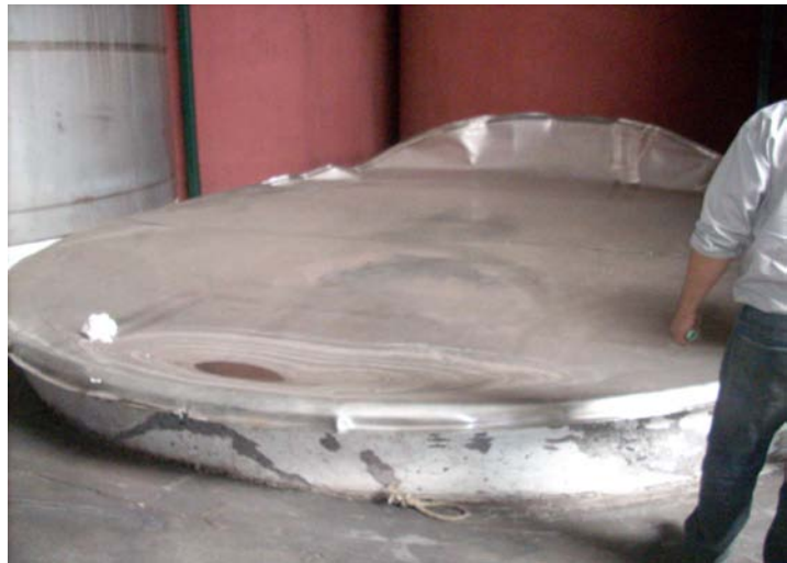
Figure 2. Failure of bottom to mantle welding of tank
