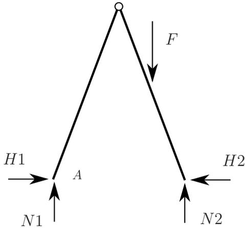
$$\begin{aligned} \Sigma V = 0 &: N_1 + N_2 = F \\ \Sigma H = 0 &: H_1 - H_2 = 0 \\ \Sigma M^A = 0 &: 2aN_2 - F(2a - x) = 0 \\ &\Rightarrow N_2 = F\left(1 - \frac{x}{2a}\right) \\ &\Rightarrow N_1 = F\frac{x}{2a} \end{aligned}$$
