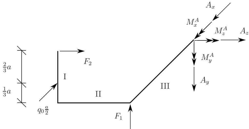
$$\begin{aligned} \Sigma F_{ix} = 0 : & & A_x &= \frac{q_0 a}{2} \\ \Sigma F_{iy} = 0 : & & A_y &= F_1 \\ \Sigma F_{iz} = 0 : & & A_z &= -F_2 \\ \Sigma M_{ix}^A = 0 : M_x^A - F_2 a = 0 & & M_x^A &= F_2 a \\ \Sigma M_{iy}^A = 0 : M_y^A + q_0 \frac{a^2}{2} - F_2 \cdot 2a = 0 & & M_y^A &= 2aF_2 - q_0 \frac{a^2}{2} \\ \Sigma M_{iz}^A = 0 : M_z^A - F_1 \cdot 2a - q_0 \frac{a^2}{6} = 0 & & M_z^A &= 2aF_1 + q_0 \frac{a^2}{6} \end{aligned}$$
