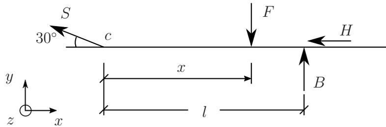
$$\sum F_x: \quad -S\cos(30^\circ) - H = 0 \quad \Rightarrow \quad \mu_0 B = -S\cos(30^\circ) \quad \Rightarrow \quad B = -\frac{1}{\mu_0} S\cos(30^\circ) \quad (\text{I})$$
