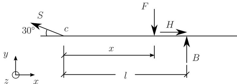
$$\sum F_x: \quad -S\cos(30^\circ) + H = 0 \quad \Rightarrow \quad \mu_0 B = S\cos(30^\circ) \quad \Rightarrow \quad B = \frac{1}{\mu_0} S\cos(30^\circ) \quad (\text{I})$$
