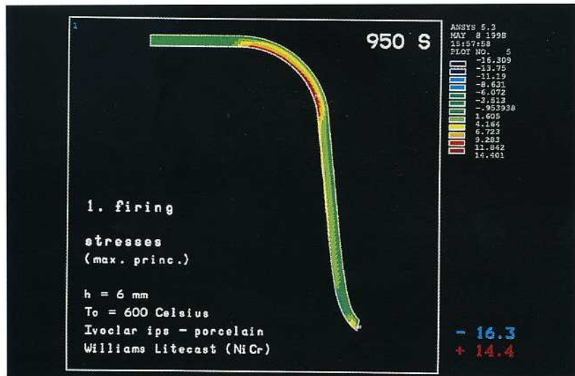
Fig 15 Distribution of residual stresses in the opaque layer.
