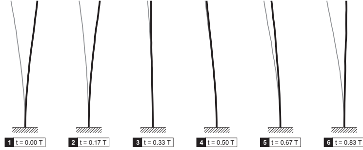
Fig. 3: Operation deflection shape during one excitation period T , f = 3.25\text{Hz} (experiment).
