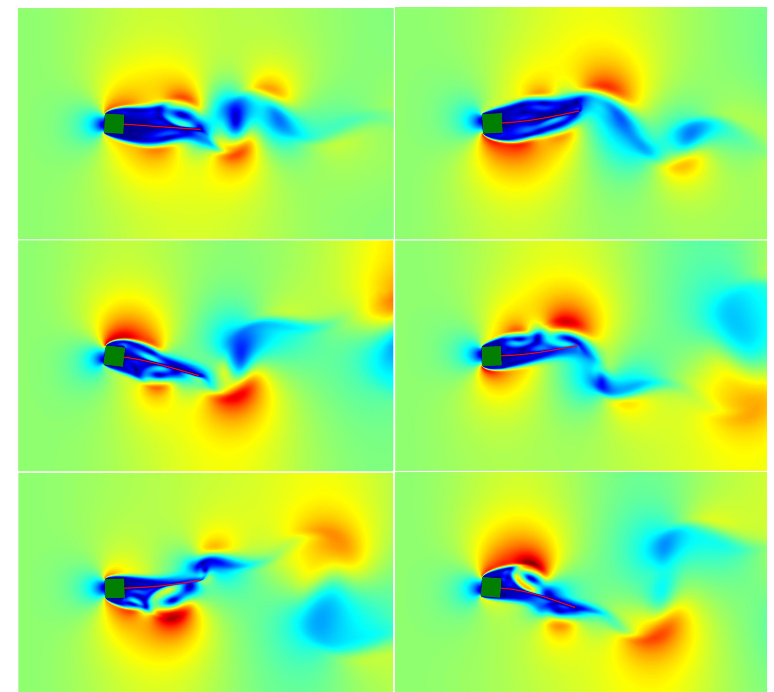
Different snapshot of the norm of the velocity field. From left to right, top to bottom:  $t = 0.5, 1, 1.5, 2, 2.5, 3$ . Colours indicate the  $L^2$  norm of the velocity field in the range of  $[0, 100]$ .
