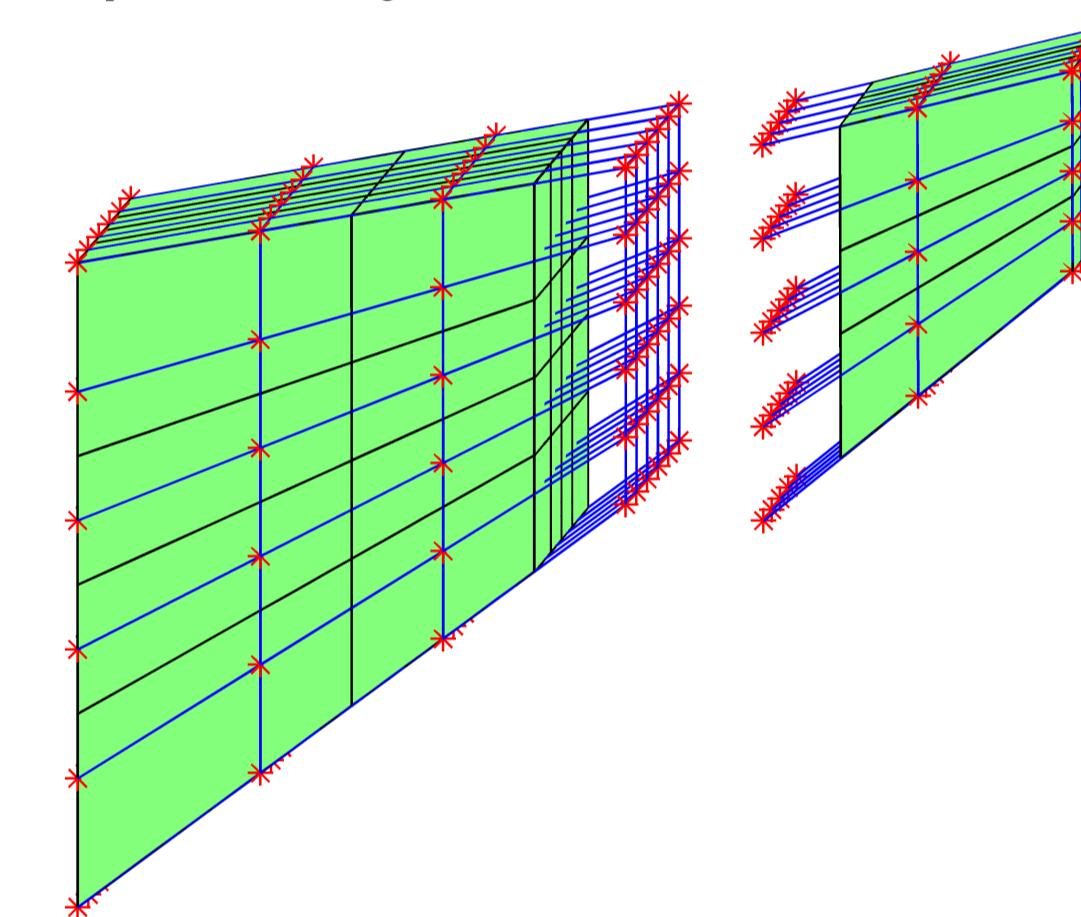
A Dirichlet boundary condition has been applied to the left surface, whereas a Neumann boundary has been applied to the right surface. Von Mises stress distribution is displayed below.
