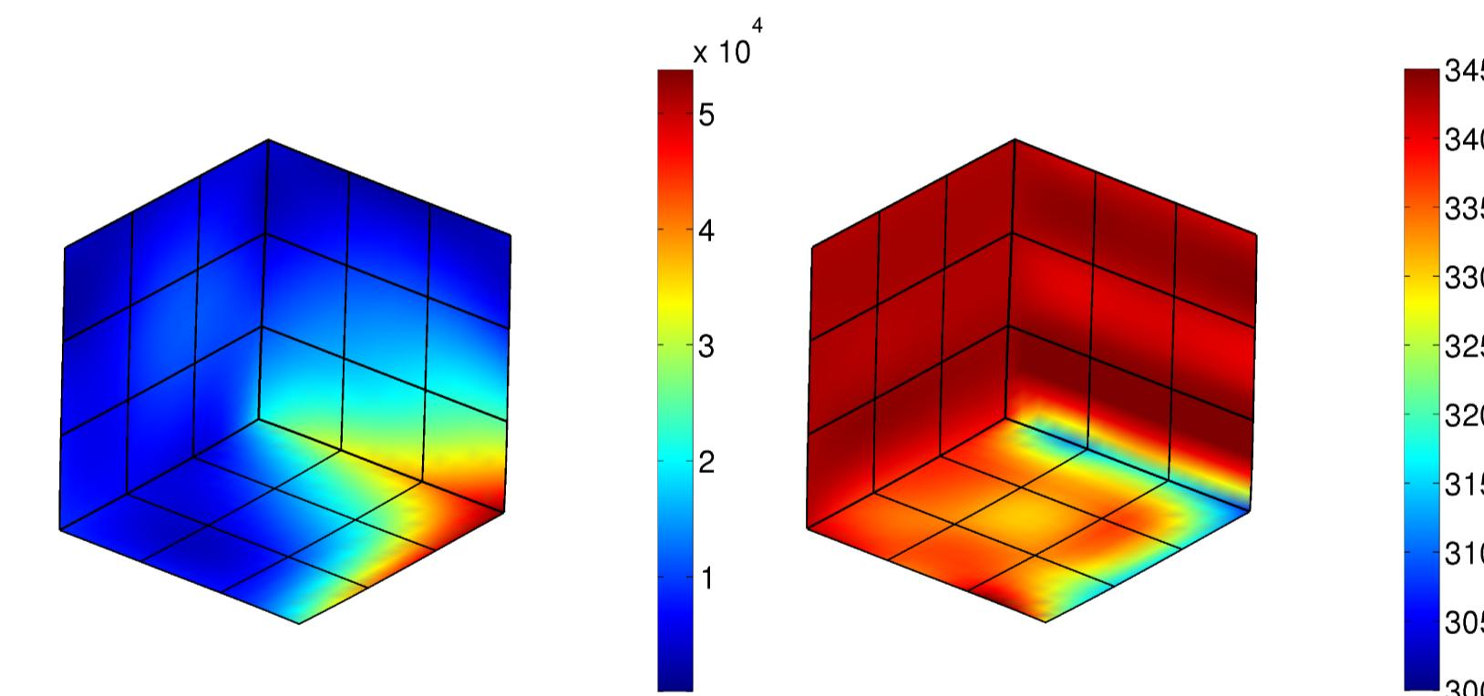
Von Mises stresses (left) and temperature (right) distribution.
