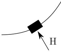
$$H = \mu \underbrace{N}_{=mg} > ma_n \quad \text{mit } a_n = \frac{v_{max}}{r}$$
