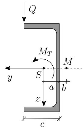
Gegeben:  $M_T = 2 \text{ kNm}$ ,  $Q = 100 \text{ kN}$ ,  $a = 2,56 \text{ cm}$ ,  $b = 2,85 \text{ cm}$ ,  $c = 8 \text{ cm}$
