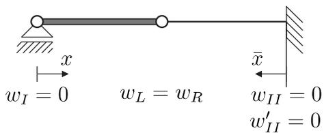
$$\begin{aligned} w_I(x=0) &= 0 \quad \Rightarrow \quad C_2 = 0 \\ w_I(x=l) &= w_{II}(\bar{x}=l) \\ w_{II}(\bar{x}=0) &= 0 \quad \Rightarrow \quad C_4 = 0 \\ w'_{II}(\bar{x}=0) &= 0 \quad \Rightarrow \quad C_3 = 0 \end{aligned}$$
