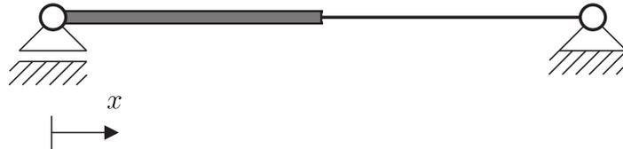
$$\begin{aligned} w_I(x=0) &= 0 & w_I(x=l) &= w_{II}(x=l) & w_{II}(x=2l) &= 0 \\ w'_I(x=l) &= w'_{II}(x=l) \end{aligned}$$
