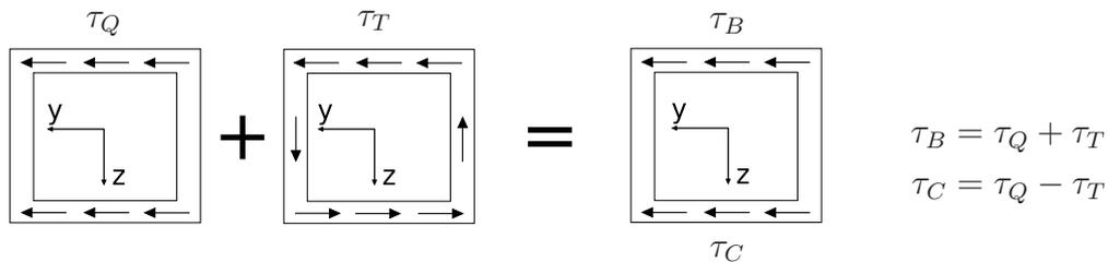
$$\begin{aligned} \tau_B &= -0,1496 \frac{N}{mm^2} - 2,370 \frac{N}{mm^2} = -2,5196 \frac{N}{mm^2} \\ \tau_C &= -0,1496 \frac{N}{mm^2} + 2,370 \frac{N}{mm^2} = 2,2204 \frac{N}{mm^2} \end{aligned}$$
