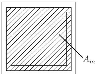
$$\begin{aligned} A_m &= \left(a - \frac{2t}{2}\right)^2 \\ &= (80mm - 5mm)^2 \\ &= 5625mm^2 \\ t_{min} &= 5mm \end{aligned}$$
