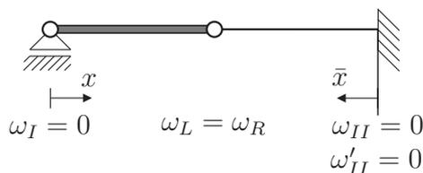
$$\begin{aligned} \omega_I(x=0) &= 0 & \Rightarrow & C_2 = 0 \\ \omega_I(x=L) &= & \omega_{II}(\bar{x}=L) \\ \omega_{II}(\bar{x}=0) &= 0 & \Rightarrow & C_4 = 0 \\ \omega'_{II}(\bar{x}=0) &= 0 & \Rightarrow & C_3 = 0 \end{aligned}$$
