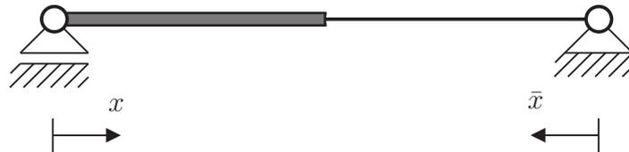
$$\omega_I(x=0) = 0 \quad \omega_L(x=L) = \omega_R(\bar{x}=L) \quad \omega_{II}(\bar{x}=L) = 0$$
