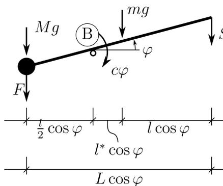
NR: Hebelarm  $mg$ :  $\left(-\frac{1}{3} + \frac{1}{2}\right)L = \frac{1}{6}L = \frac{1}{6} \cdot \frac{3}{2}l = \frac{1}{4}l$
