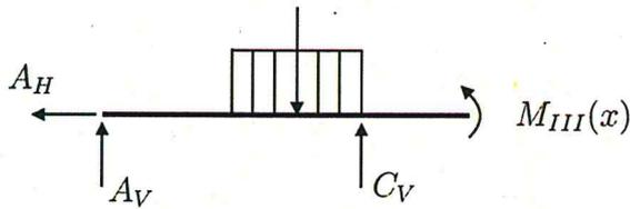
$$\begin{aligned} \sum M^x = 0: \quad & M_{III}(x) - C_V \cdot (x - 2a) + q_0 \cdot a \left(x - \frac{3}{2}a\right) - A_V \cdot x = 0 \\ \Rightarrow M_{III}(x) = & \frac{5}{4} q_0 a (x - 2a) - q_0 a \left(x - \frac{3}{2}a\right) - \frac{1}{4} q_0 a \cdot x \\ = & \frac{1}{4} q_0 a \cdot x - \frac{10}{4} q_0 a^2 + \frac{3}{2} q_0 a^2 - \frac{1}{4} q_0 a \cdot x \\ = & -q_0 a^2 \quad + \end{aligned}$$
