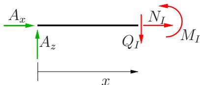
$$\begin{aligned} \sum F_{ix} = 0 : N_I(x) &= -A_x = qa \\ \sum F_{iz} = 0 : Q_I(x) &= A_z = \frac{1}{2}qa \\ \sum M^B = 0 : M_I(x) &= A_z x = \frac{1}{2}qax \end{aligned}$$
