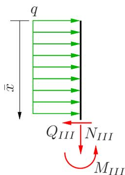
$$\begin{aligned} \sum F_{ix} = 0 : N_I(\bar{x}) &= 0 \\ \sum F_{iz} = 0 : Q_I(\bar{x}) &= q\bar{x} \\ \sum M^B = 0 : M_I(\bar{x}) &= q\frac{\bar{x}^2}{2} \end{aligned}$$
