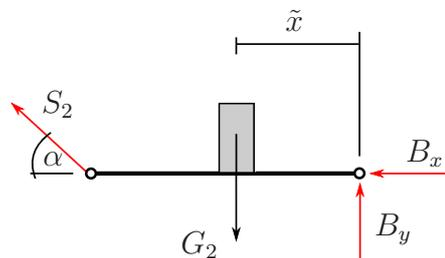
$$\begin{aligned}\sum M^b = 0 : \quad & -S_2 \cos(\alpha) l + G_2 \tilde{x} = 0 \\ \Rightarrow S_2 &= G_2 \sqrt{2} \frac{\tilde{x}}{l}\end{aligned}$$
