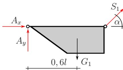
$$\begin{aligned}\sum M^A = 0 : \quad & S_1 \cos(\alpha) l - 0,6 G_1 l = 0 \\ \Rightarrow S_1 &= \frac{3\sqrt{2}}{5} G_1\end{aligned}$$
