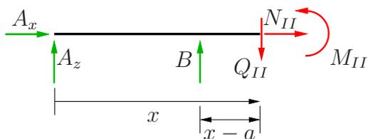
$$\begin{aligned} \sum F_{ix} = 0 : N_{II}(x) &= -A_x = qa \\ \sum F_{iz} = 0 : Q_{II}(x) &= A_z + B = -qa \\ \sum M^B = 0 : M_{II}(x) &= A_z x + B(x - a) = -qax + \frac{3}{2}qa^2 \end{aligned}$$
