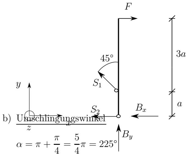
$$\begin{aligned} \sum M_z^B = 0 : \quad S_1 \cdot \frac{\sqrt{2}}{2} \cdot a - F \cdot 4a &= 0 \\ \rightarrow S_1 &= 4\sqrt{2}F \end{aligned} \quad (1)$$
