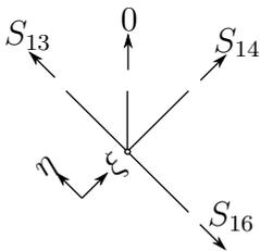
$$\begin{aligned} \sum F_{i\xi} = 0 &\rightarrow S_{14} = 0 \\ \sum F_{i\eta} = 0 &\rightarrow S_{13} = S_{16} \end{aligned}$$
