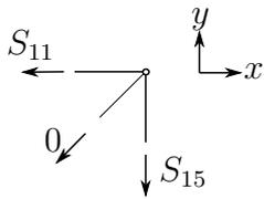
$$\begin{aligned} \sum F_{ix} = 0 &\rightarrow S_{11} = 0 \rightarrow S_{10} = 0 \\ \sum F_{iy} = 0 &\rightarrow S_{15} = 0 \end{aligned}$$
