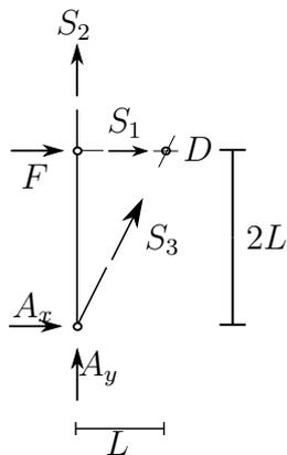
$$\begin{aligned} \sum M_i^{(A)} = 0 &: F \cdot 2L + S_1 \cdot 2L = 0 \rightarrow S_1 = -F \\ \sum M_i^{(D)} = 0 &: S_2 \cdot L + A_y \cdot L - A_x \cdot 2L = 0 \\ &\rightarrow S_2 = -(F + 2q_0L) \end{aligned}$$
