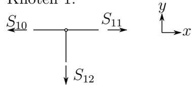
$$\begin{aligned} \sum F_{iy} = 0 &\rightarrow S_{12} = 0 \\ \sum F_{ix} = 0 &\rightarrow S_{10} = S_{11} \end{aligned}$$
